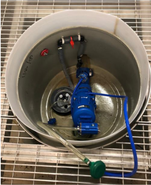
The valve pit was filled with water to a depth that was 300mm (11.8") over the controller
